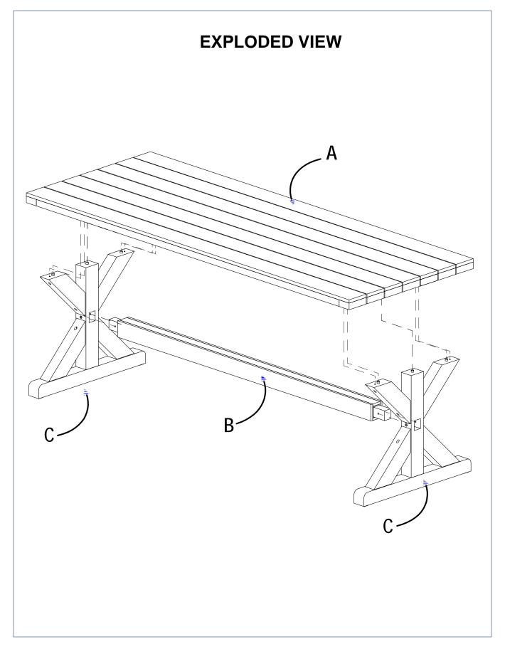
STEP 1: Inserts Screw 7x45 (E) From Legs Frame (2xC) into Cross Beam. And use Allen key (F) to secure.
