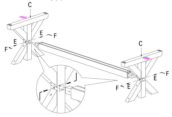
STEP 2: Insets Screw 7x70 (D) From Leg (2xC) Step 1 into Top Table. And use Allen key (F) to secure.
